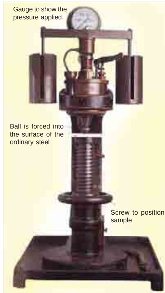
Brinell Tester : Hardness can be defined as the resistance of a metal to attempts to deform it. This machine invented by the Swedish metallurgist Johann August Brinell (1849-1925), measure hardness precisely.
